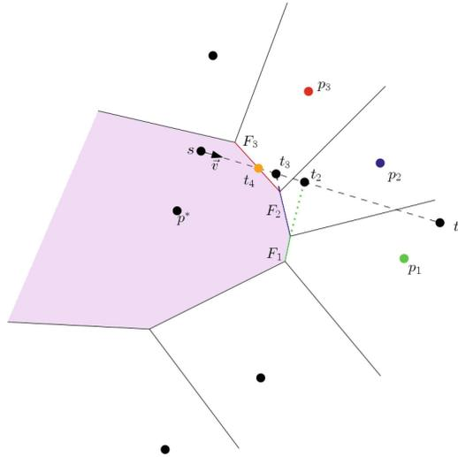
**Fig. 3.** An example of the boundary oracle converging to a solution. The query ray is  $r = (s, v)$  and  $t_4 = r \cap \partial P$  is the solution.  $t_1, t_2, t_3, t_4$  were computed in sequence.
