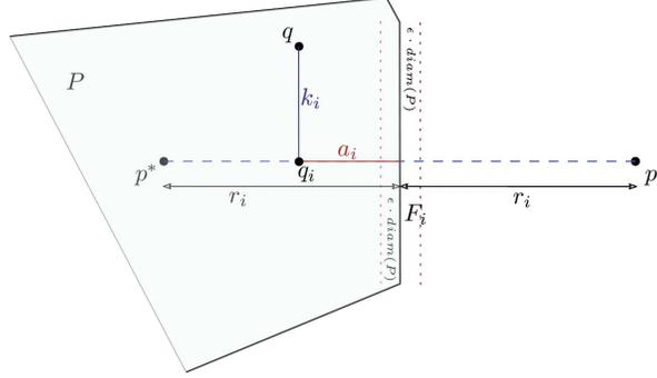
**Fig. 2.**  $p_i$  corresponds to the symmetric point of  $p^*$  about the facet  $F_i$ . We decompose the distances  $\|p^* - q\|_2$  and  $\|p_i - q\|_2$  and express them in terms of  $a_i$  and  $k_i$ . Notice how  $q \in P^{-\epsilon} \Rightarrow a_i \geq \epsilon \cdot \text{diam}(P)$  and how  $k_i < \text{diam}(P)$ , as  $q$  cannot be a vertex.
